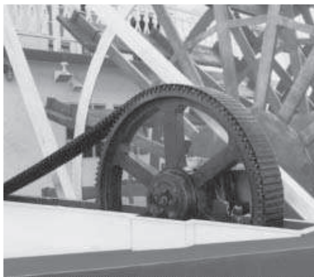
Paddle wheel drive on a large riverboat
